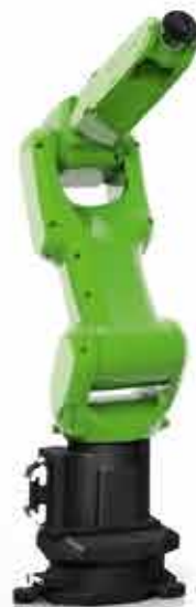
CR-7iA/L Payload: 7 kg Reach: 911 mm
