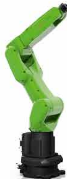
CR-14iA/L Payload: 14 kg Reach: 911mm
